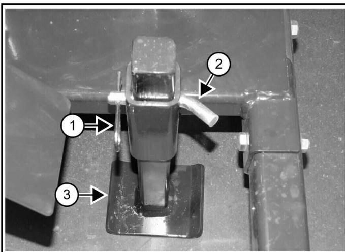
1. Remove the retaining pin (Item 1) and the pin (Item 2) [Figure 18].
