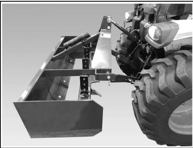
3. Raise the implement to the travel position [Figure 32]. See the compact tractor Operation & Maintenance Manual for detailed information on operating the three-point hitch.
