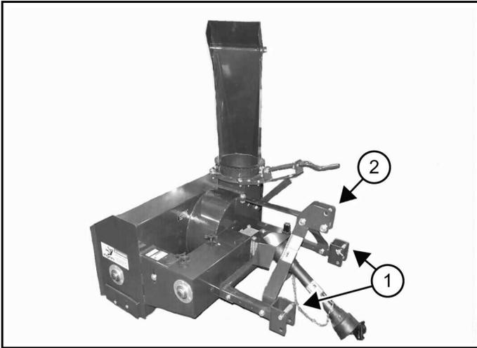
Inspect the lower three-point mounts and lower mounting pins (Item 1) and upper three-point mount and pin (Item 2) [Figure 6], along with all welds on the three-point snowblower for wear and damage each time the three-point snowblower is removed from the machine.
