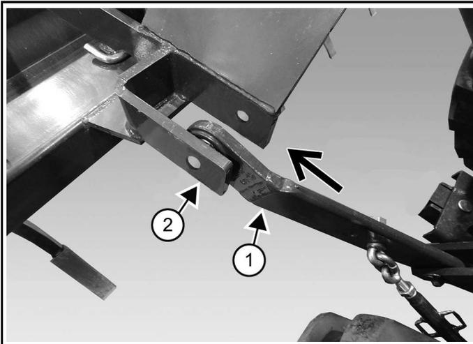
5. Drive the compact tractor to the implement and align the lower links (Item 1) with the implement lower mounts (Item 2) [Figure 11] (both sides).
