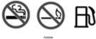
Stop the engine and let it cool before adding fuel. No smoking! Do not refuel a machine near open flames or sparks. Fill the fuel tank outdoors.
