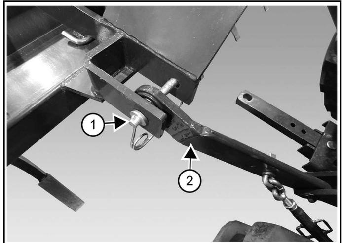
8. Install the lower implement pin (Item 1) through the lower mounts and lower link (Item 2) [Figure 12] (both sides) and secure with retaining clip.
